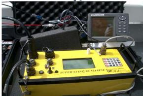
The **SuperSting R8 Marine** instrument continuously records and stores data from a GPS receiver. Current is injected every 3 seconds and 8 apparent resistivity values representing 8 depth levels are read for each current injection. Our modeling software EarthImager 2D has a Continuous Resistivity Profiler (CRP) option to process these data. The system comprises the SuperSting Marine, the Marine Log Manager software and an electrode towing cable.
