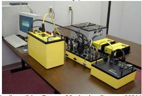
The **SuperSting Remote Monitoring System** (SSRMS) is designed for unattended monitoring applications on landfills, well sites, dams and other locations where changes of resistivity conditions over time need to be recorded and analyzed. The electrodes can be installed at the surface or in boreholes. An Internet connection for the server PC, preferably in the form of a DSL broadband connection, allows communications between the remote equipment and the main office.
