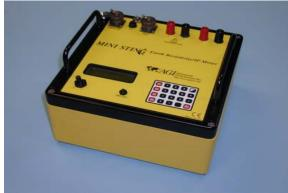
The **MiniSting** is a low cost, single channel, memory earth resistivity and IP instrument mainly designed for manual measurements with four electrodes, but can also be equipped with automatic electrodes.
