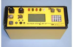
The **SuperSting R8/IP** is a state-of-the-art 8-channel portable memory earth resistivity meter with memory storage of readings and user defined measurement cycles. It provides the highest accuracy and lowest noise levels in the industry. It can be used with our patented Multi-channel Swift Dual Mode Automatic Multi-electrode cable (patent 6,404,203) or with different capability switch boxes and passive cables to form a system ideal for 1D, 2D or 3D resistivity or IP measurements.
