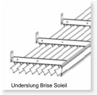
As the name implies Underslung/Overslung refers to the position of the extruded aluminium blades in relation to the supporting rafters.
