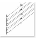
Vertical Brise Soleil refers to the framing supporting the aluminium blades. The elliptical blades & austere lines add to the architectural aspect of the design.
