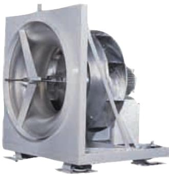
The standard Air Handling Unit Fan Section contains a double inlet double width fan with either multiblade forward curved, backward curved or backward curved areofoil bladed impellers. Alternative fans are available.
