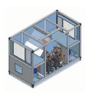
Recuperators are of the high efficiency type formed from aluminium plates with a galvanised steel casing. Plates are sealed to prevent cross contamination. The recuperator is utilised during the summer months to provide "free cooling".
