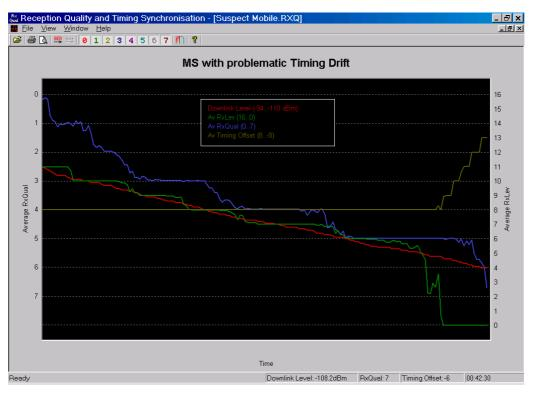
Fig. 1: RxQual, RxLev and Timing response to level change against time
