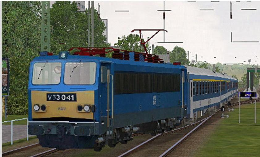
The ‘Gigant’ is a Co-Co electric locomotive with thyristor rectifiers introduced in the mid-eighties for fast and heavy passenger trains and heavy freight trains. Ten have been upgraded for 160 km/hr work and renumber in the V63.100 series. V63.106 was downgraded. However, as they cannot sustain 160 km/hr EC trains to Wien used Austrian locos equipped for working in Hungary.
