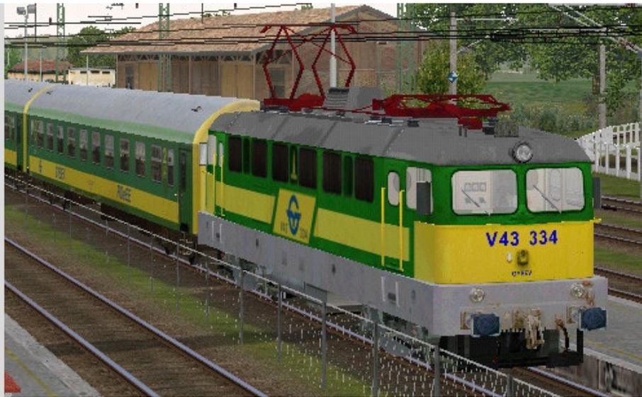
The main Electric motive power in Hungary. Designed by a consortium including Krupps and Alstom to meet a specification of MAV, with most assembled and built in Hungary. The original bogies damaged poor track, so most have been rebuilt with new rubber suspension, and 30 have been modified for push-pull operation and the central closing of the doors. These are renumbered as V43.2360 and have a new livery.
