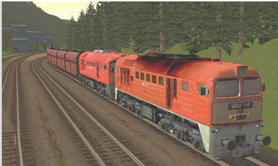
The ‘Szergej’ Co-Co diesel built in the Soviet Union for standard gauge. Hungary would have preferred more of the Swedish built NOHAB of which they had 20, as a steam replacement, but were essentially forced to take the inferior M62 (in terms of reliability, noise and fuel and oil usage). Designed for freight, it had no passenger heating, so a separate wagon with a steam boiler, and later a diesel generator, were used to heat the passenger cars. Used for Passenger, and freight.
