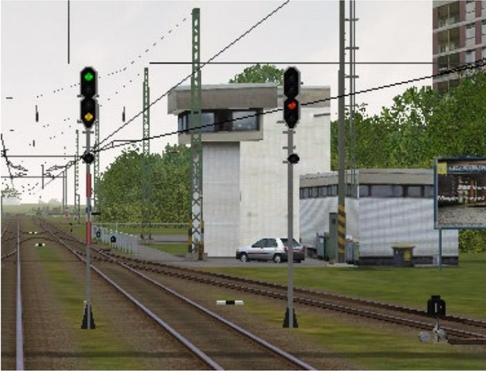
Hungary uses a block signal system of four lights (Green, yellow, red, yellow) to signal the speed of the train in the current, and in the next block.
