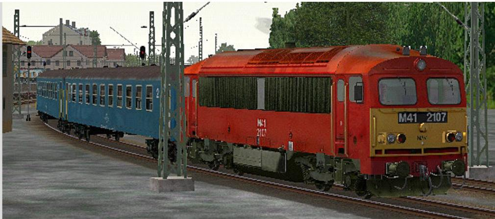
Developed by Ganz from a design for the Greek Railways as a passenger engine with low axle loads for branch lines. Class M41 "Rattler" is diesel hydraulic" powered by a SEMT-Pielstick designed V12 engine. It contains a train-heating generator. The loco is underpowered for hauling more than 6-8 coaches
