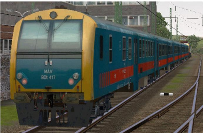
Modernised push pull stock. The stock with the red bands has only UIC connections for use with the modernized V43.
