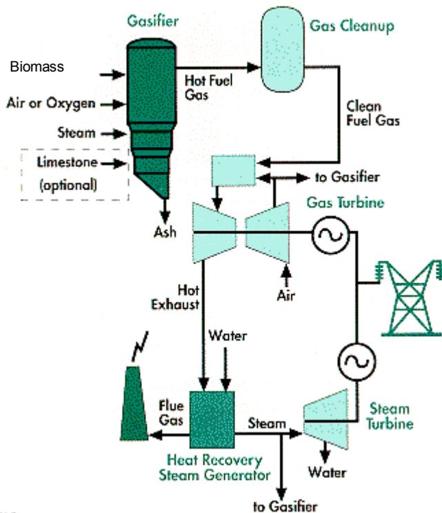
**Figure 1. Integrated Biomass Gasification Combined Cycle Power Generation Concept.**
