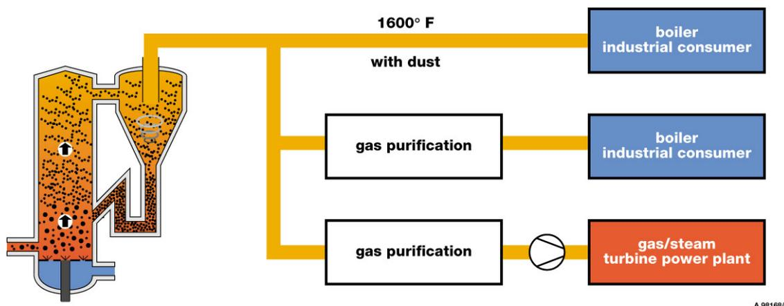
**Figure 5. Typical uses of the Biomass Gasification Concept.**
