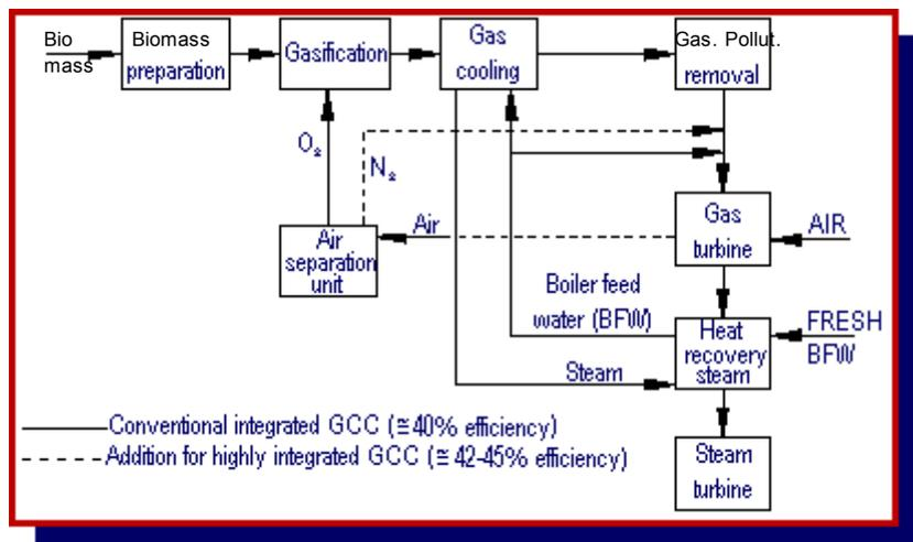
**Figure 7. IBGCC Process Flow.**
