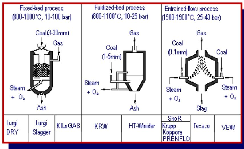
Figure 3. “Direct” Gasification Processes.
