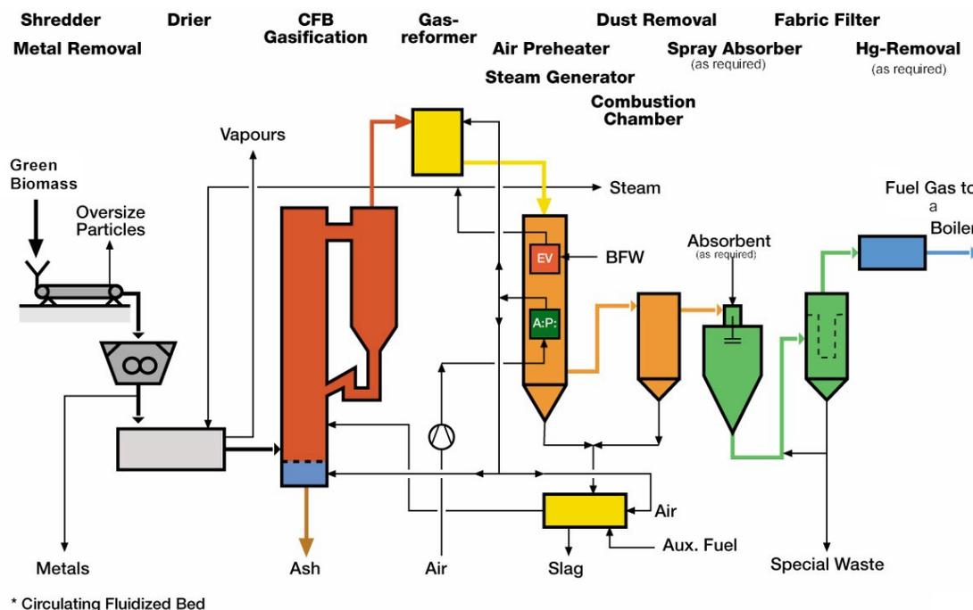
**Figure 2. Typical Biomass Gasification System Schematic.**
