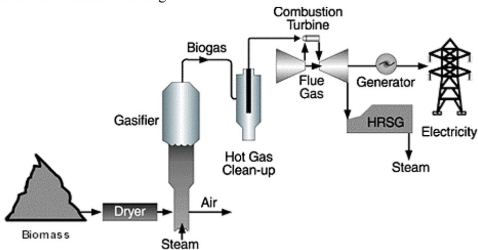
**Figure 9. Simplified IBGCC Schematic**
