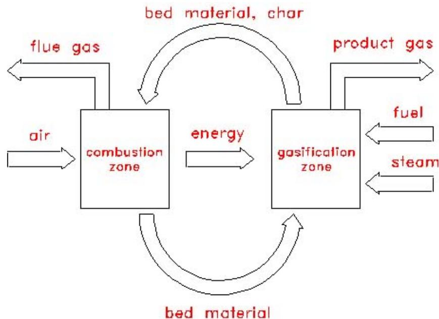
**Figure 6. Basic idea of the gasification process.**
