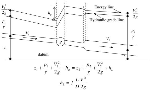
Friction factor f is a function of Reynolds number  $(R_N)$  and relative roughness  $(k_s/D)$ . It can be found from Moody's diagram or Colebrook equation:
