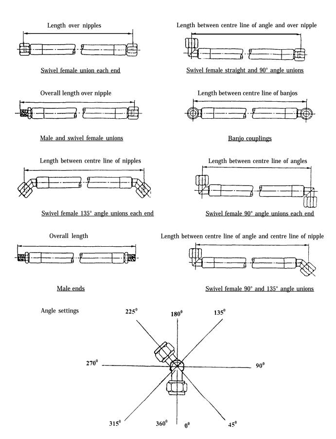
Fig 1 Method of Dimensioning Flexible Hose Assemblies
